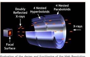
Illustration of the design and functioning of the High Resolution Mirror Assembly (HRMA) on Chandra. X-rays that strike a mirror head-on are absorbed, while X-rays that hit a mirror at grazing angles are reflected like a pebble skipping across a pond. Thus, X-ray telescope mirrors are shaped like barrels rather than dishes, where the X-rays reflect off the inner, polished surfaces and are focused onto a detector to produce an image.
