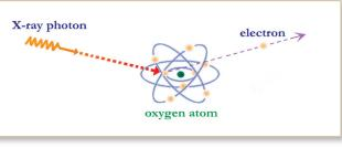
The energy of the X-ray goes tearing into one of the electrons away from its orbit around the nucleus of a nitrogen or an oxygen atom.
